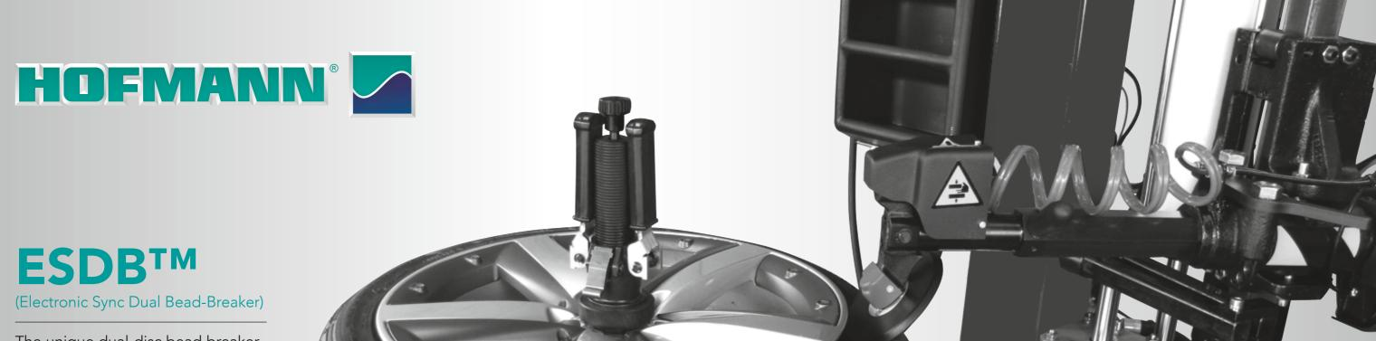
The unique dual-disc bead breaker with servo drive. Bead breaking in an upright position: faster, easier, ergonomic and effortless. The bead roller is applied to detach both soft and stiff beads.
