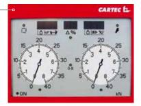
The measuring range for both version is 0–8 / 0–40 kN, when a car is tested, the measuring range switches automatically to 8 kN.
