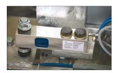
The features to be tested are detected by means of well-proven strain-gauge type load cells.
