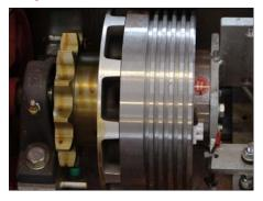
During testing the rolling resistance is simulated with an eddy current brake integrated in the bench.
