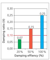
Damping ratios & determined with suspension tester FWT 3800 on shock absorbers having different damping efficiencies; the ratios were determined on a car under in-situ conditions.
