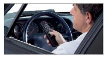
The radio remote control unit can be used to control the testing equipment from driver's seat at the entire discretion of the operator, e.g. by starting the brake tester only, or by conducting the tests in the sequence he prefers.
