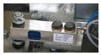
The features to be tested are detected by means of well-proven strain-gauge type load cells. This wear-free measuring system ensures reliable and error-free measurement of the forces produced.
