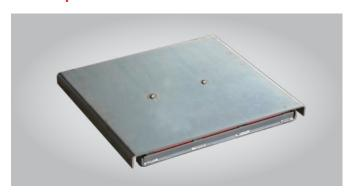
The side-slip tester is designed to measure toe of the vehicle under test immediately. No additional tests are necessary as the testing plate is positioned directly in front of the suspension or brake tester and the vehicle simply rolls over. The data automatically detected supplies a sound diagnostics of toe-in and toe-out. The measured value is read out in 0 +/- 20 mm/m.
