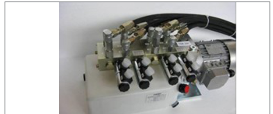
Hydraulikaggregat / hydraulic aggregate
